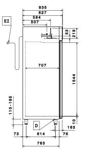
ED Remote electrical connection RO Refrigerant Outlet ΕI Electrical inlet (power) Refrigerant Inlet
